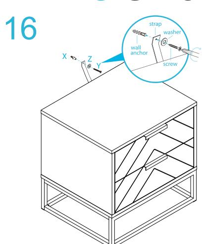
Once assembled lift furniture into place, do not drag. Use a drill to create a small hole lining up with the top of the safety strap (V). Fasten to the wall using 1x washer (Z), 1x wall anchor (X) and 1x wall screw (Y). Ensure unit is balanced and steady before use. You're done, enjoy!
