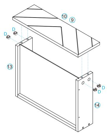
Attach panels [9]/[10] to panels [13] and [14] secure with 8x locking nuts (D). Tighten with a screwdriver.
