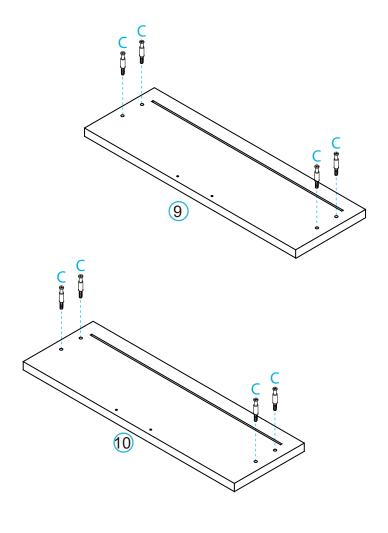
Insert 8x bolts (C) into panels [9]/[10]. Tighten with a screwdriver.
