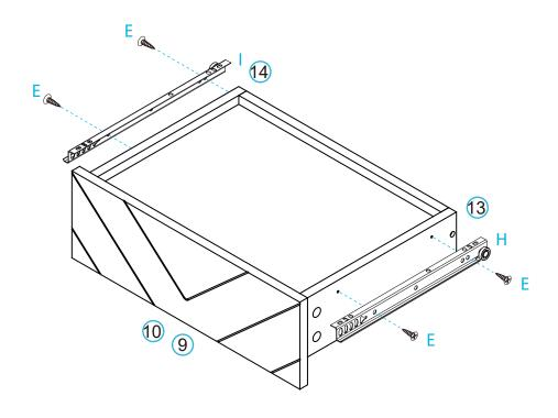
Attach slide rail (I) and slide rail (H) to the underside of the side panels as shown. Secure with 8x screws (E) and tighten with a screwdriver.
