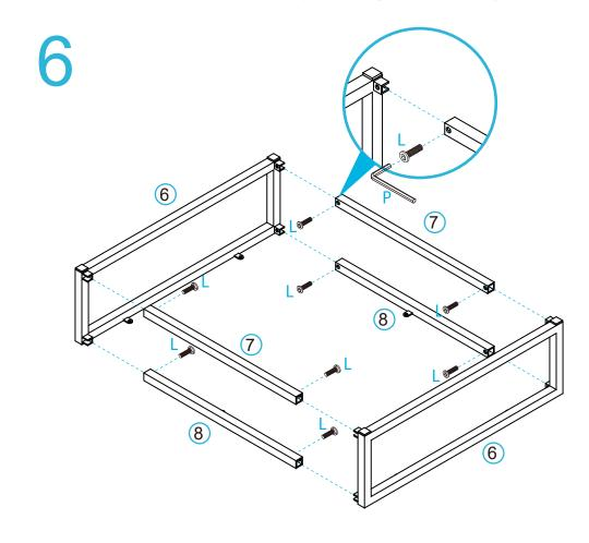
Attach panels [6] to panels [7] and panels [8] with 8x bolt (L). Tighten with an Allen Key (P).
