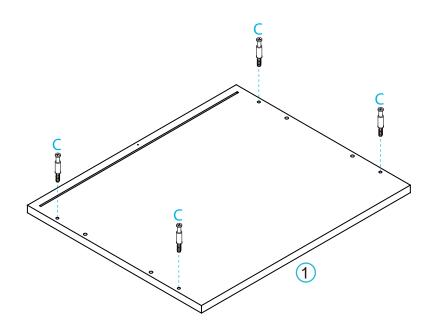
Insert 4x bolts (C) into panel [1] and tighten with a screwdriver.
