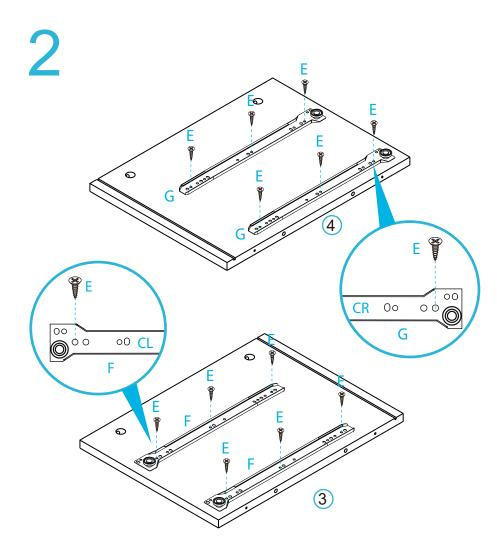
Attach 2x slide rails (F) and 2x slide rails (G) to panels [3] and [4] as shown and secure with 12x screws (E). Tighten with a screwdriver.
