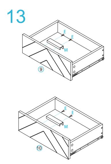
Attach 2x handles (M) to panels [9]/[10] and secure with 4x screws (E). Tighten with a screwdriver.
