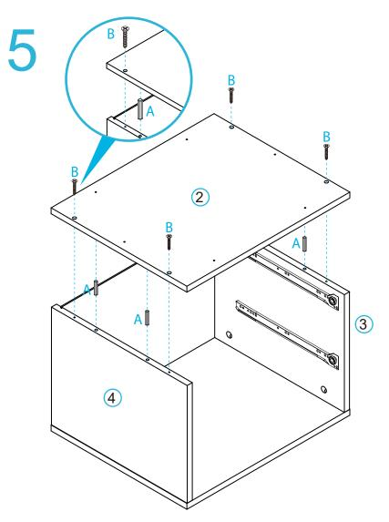
Attach panel [2] to the unit with 4x dowels (A) and secure with 4x screws (B). Tighten with a screwdriver.
