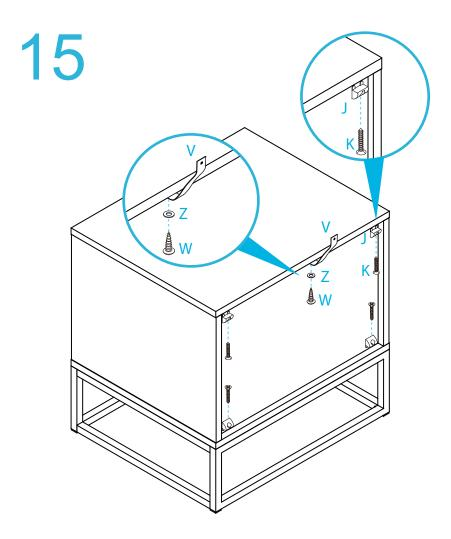
Attach 4x wedges (J) into the corners of the back of the unit and secure with 4x screws (K). Tighten with a screwdriver. Attach 1x safety strap (V) to the top of the back side of the unit as shown using 1x washer (Z) and 1x screw (W). Tighten with a screwdriver.
