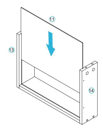
Attach panels [12], [13] and [14] as shown using 8x screws (O). Tighten with a screwdriver.
