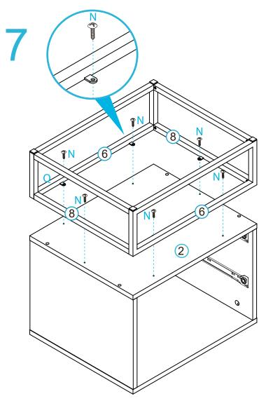
Attach panels [6] to panel [2] with 6x small screw (N). Tighten with a screwdriver.
